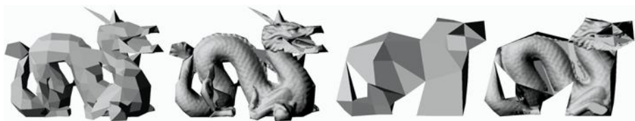
Fig. 6. Left two: flat-shaded and normal mapped dual contour surface (558 quads). Right two: flat-shaded and normal mapped dual contour surface (65 quads).
