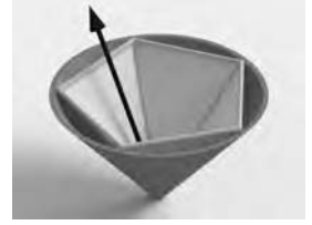
Fig. 1. Linearized friction cone (5 edges)
