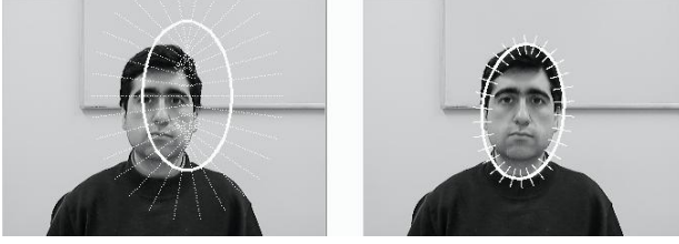
Fig. 2. Contour model fitting to the head boundary, before and after 12 steps of CCD optimization. Sample points used by the algorithm are shown.
