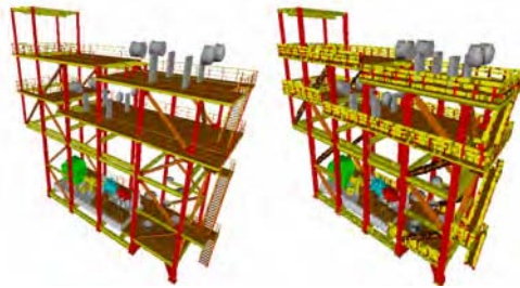
Fig. 1. Thin objects: ( left ) represented as geometry, ( right ) represented as voxels, causing visual artifacts
