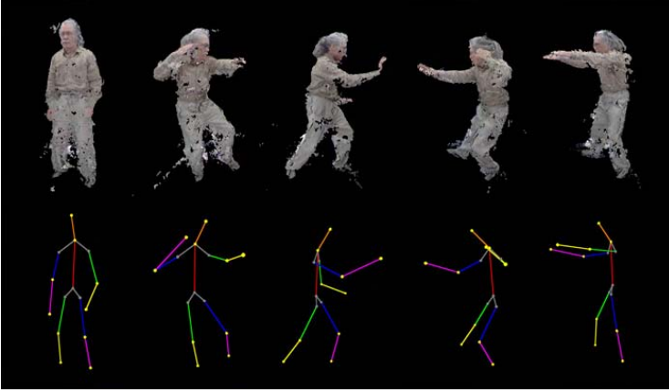
Fig. 3. Top: Stereo reconstruction of our tele-immersion system. Bottom: Real-time skeleton extraction from 3D point cloud data.
