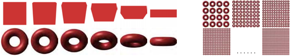
Fig. 5. Left: Several viewing-angles used for testing torus rendering performance (see Table 1). In the first row the bounding-box used for our GPU primitive, in the second row the torus itself. Right: Rendering multiple tori for the results in Figure 6.
